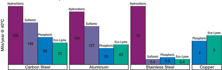
Comparative Corrosion Rates of Common Descaler Chemistries
