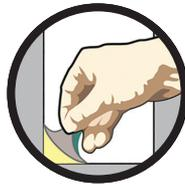
2. Remove white backing tape to expose the sticky resin. Apply patch to repair area with sticky side down and press firmly to make sure that patch seals the entire area.
