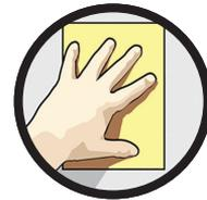
3. Remove the film backing on top side and expose to UV or sunlight. Curing time depends on UV intensity, between 5 minutes (sunny) and 50 minutes (cloudy) or use Nu-Calgon UV flashlight/glasses kit (p/n: 4050-15) when curing indoors.
