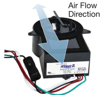
4. The iWave-R has universal voltage capability, connect 24VAC to 240VAC voltage input, whatever is most convenient for quick installation. Although the device only pulls 10 watts, sometimes a dedicated 24VAC power supply may be necessary depending on the current load on the transformer for other system accessories.
