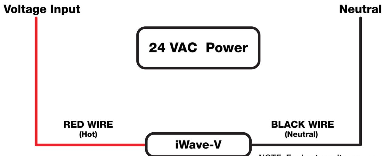
**NOTE:** For best results, power continually. From time-to-time, lint/dust must be brushed off the iWave-V emitters with a soft bristle brush. Turn off system first.
