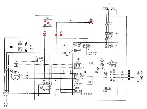
Remove run compressor connection from RUN (RD) and tie the compressor to the SureStart's [1] Connect [2] to RUN (RD).
