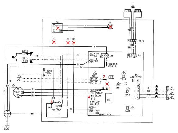
Remove red wire connection at L1 and tie it to the SureStart's [1] Connect [2] to L1.
